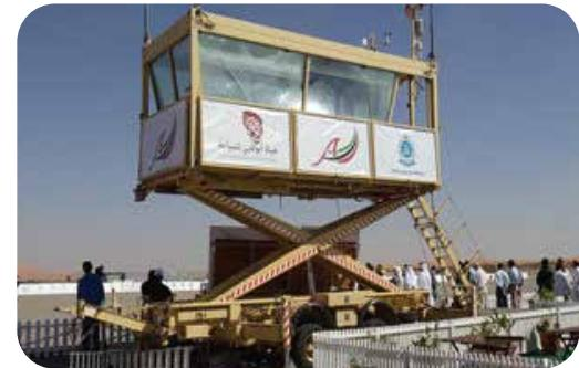
The ability to deploy towers remotely and on site at any event provides a professional operational working environment for our well trained staff to provide Air Traffic and Aviation Support services at events throughout the United Arab Emirates.
